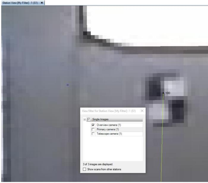
13. Check the deviation of the point to the object center, 3 pixels is OK. Here the deviation is approximately 1.8 pix which is acceptable.
